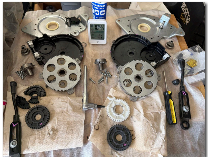
Convertible top transmissions and arms all cleaned up and ready for reassembly
