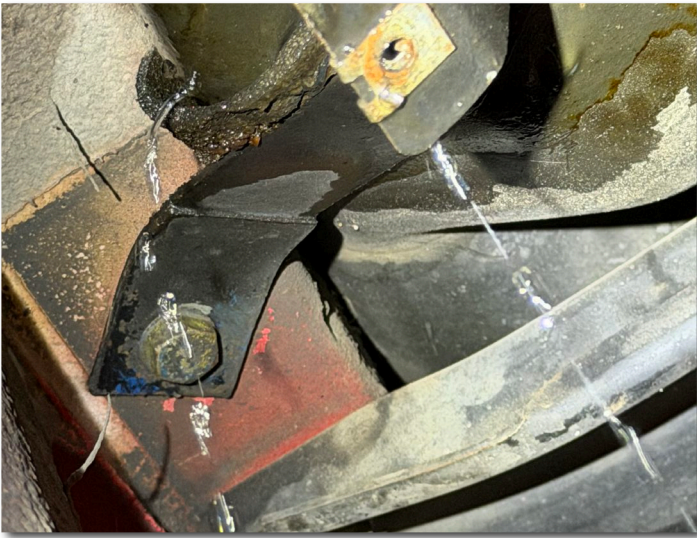
The leaking fuel tank.
