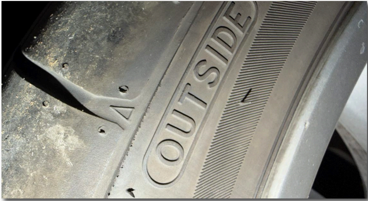
The Even on the Cayenne's tire the triangle is there to help measure sidewall roll over.
