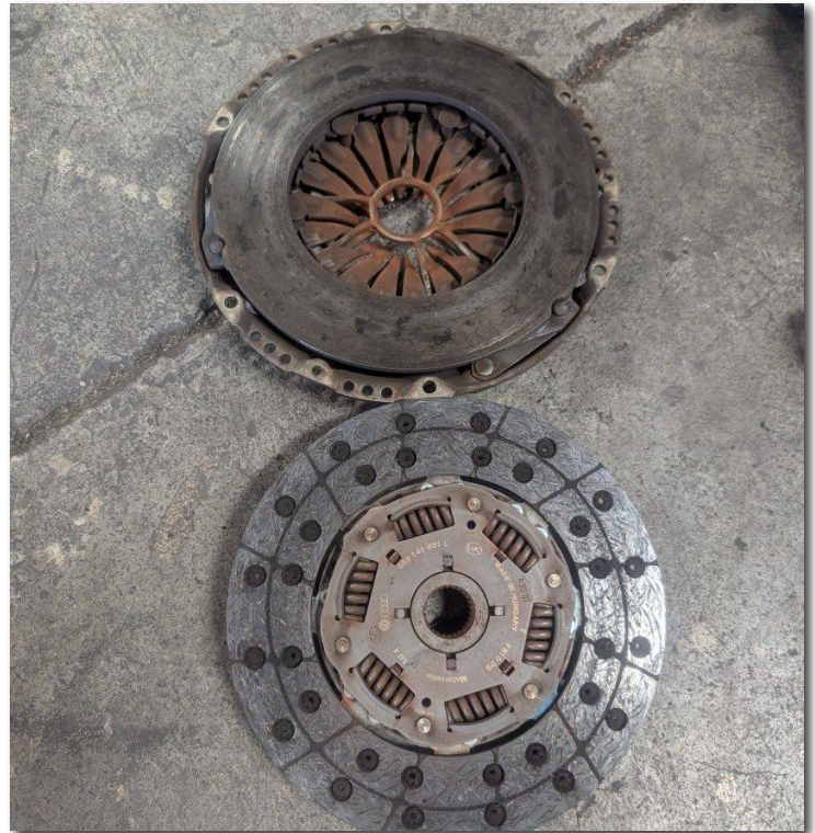
Clutch assembly doesn't look too bad for all the miles and heavy loads.
