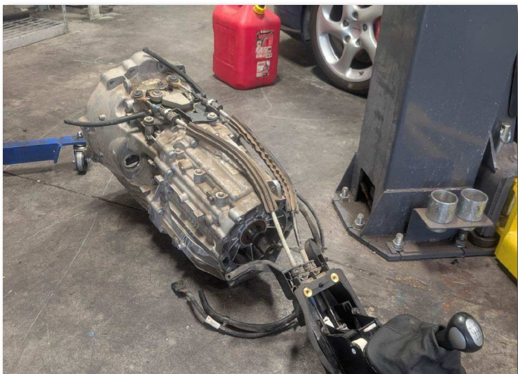
The manual transmission out of a V8 Cayenne. Not a common sight - there are reports that fewer than 350 manual Cayenne GTS vehicles were built.
