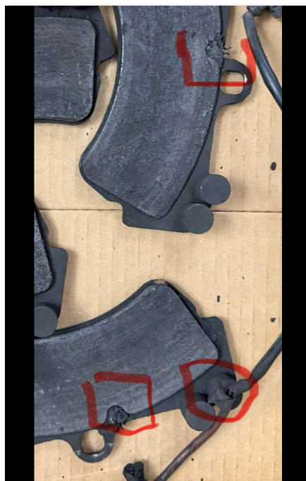
Brake sensors melted beyond functionality.
