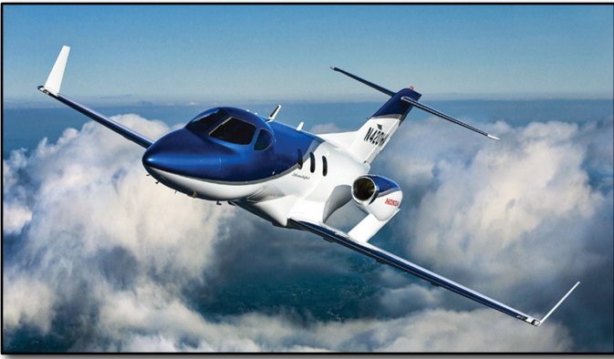
The innovative HondaJet with pylon mounted engines - Credit: Blog.privatefly.com (noted in references)
